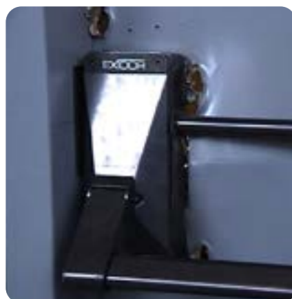
Inside view after 10 mins and the 4th bolt is still holding the door secure.
