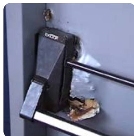
Inside view after 15 mins and the 4th bolt is still holding the door secure.
